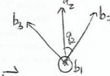
$${}^A\vec{w}^C = -\dot{q}_2 \vec{b}_1 + (\dot{q}_1 cq_2) \vec{b}_2 + (\dot{q}_3 + \dot{q}_1 sq_2) \vec{b}_3$$
