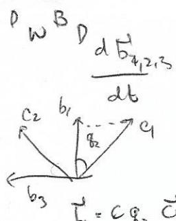
$$\vec{b}_1 = c_{q_2} \vec{a}_1 + s_{q_2} \vec{a}_2$$
