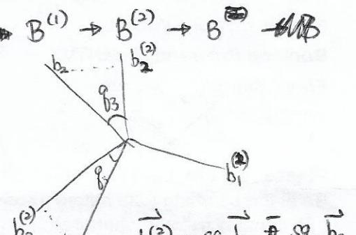
$$\begin{aligned} {}^N\vec{\omega}^B &= {}^N\vec{\omega}^A + {}^A\vec{\omega}^B \\ &= \dot{q}_1 \vec{a}_1 + \dot{q}_2 \vec{b}_2^{(2)} + \dot{q}_3 \vec{b}_1 + \Omega \vec{a}_3 \end{aligned}$$
